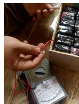
Figure 7c: voltage measurement on product
