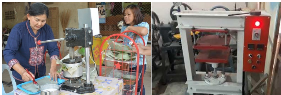
Figure 2 Machine for forming natural banana leaves using hand pressure of Sukhothai and mechanical packaging forming machine
