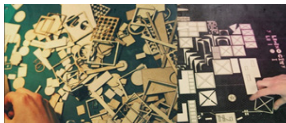
Figure 6: Laser cuttings made for items that requires intricate details. (The Making of Lumino City, 2016)
