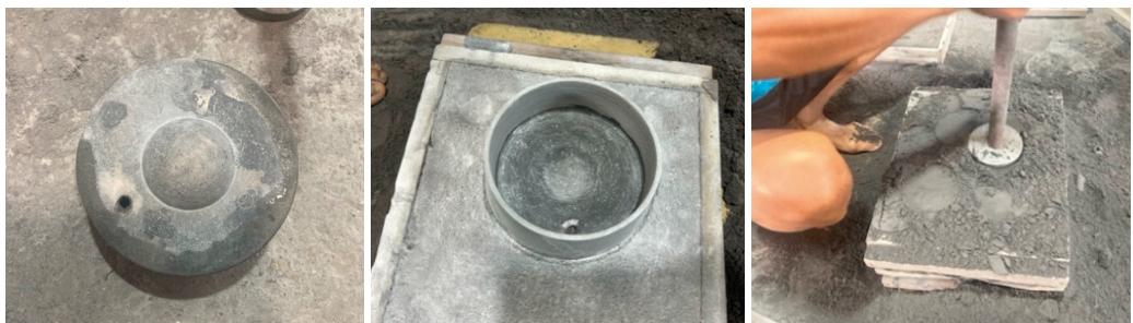
Figure 5. Shaping the Gong Mold with Precise Measurements
