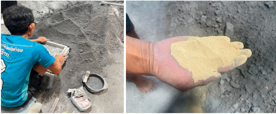
Figure 4. Preparing Clay and Ash Mixture for Mold Making
