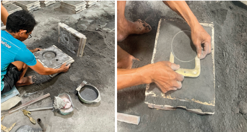
Figure 6. The Formation of the Central Core Using a Clay and Ash Mixture, Similar to the Base Mold Preparation
