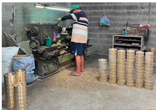
Figure 9. Polishing and Lathe Processing to Smooth the Gong Surface, Enhancing Acoustic Quality and Aesthetic Appeal
