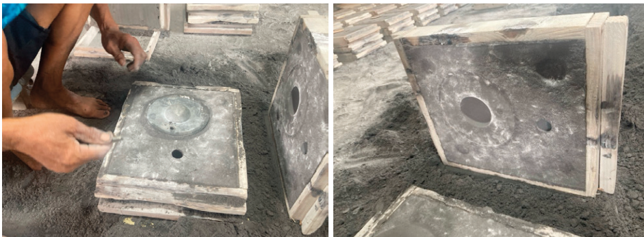
Figure 7. Forming the Gong Knob Using Clay Mixture to Create the Central Protrusion, Ensuring Precision in Size and Height
