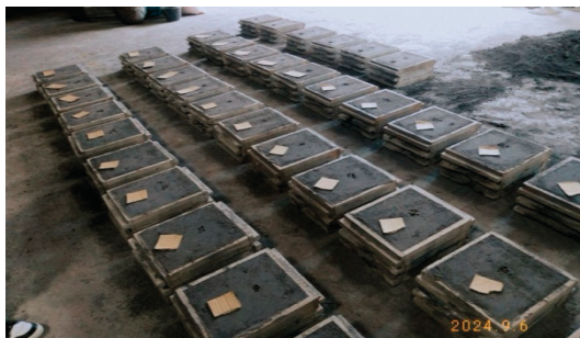
Figure 8. Drying the Completed Mold in a Well-Ventilated Area
