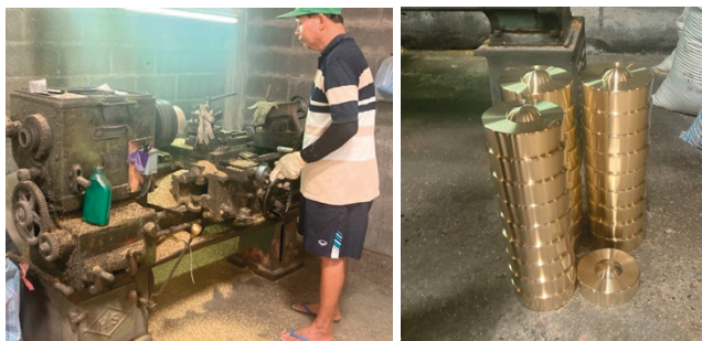
Figure 10. Polishing and Lathe Processing of the Gong Surface after Mold Removal to Achieve Smoothness and Shine
