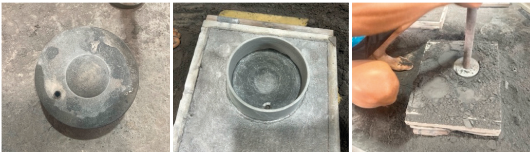
Figure 5. Shaping the Gong Mold with Precise Measurements
