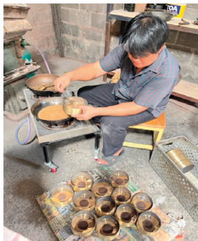
Figure 11. Applying Lead and Wax Mixture onto the Gong Knob for Sound Tuning and Resonance Adjustment
