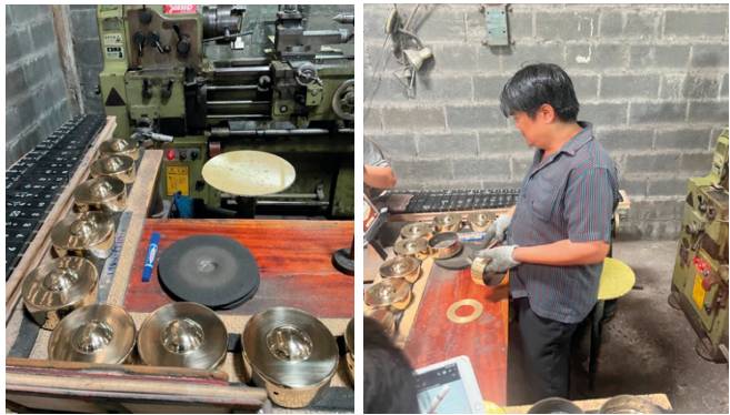
Figure 12. Fine-Tuning the Gong Sound to Achieve the Desired Pitch and Resonance Using a Tuner and Traditional Listening Techniques
