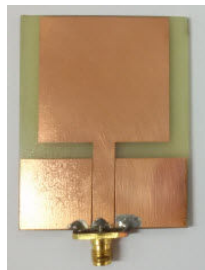
Figure 4 The Monopole aerial with square shape which related to the horizontal transmission line and the response.
