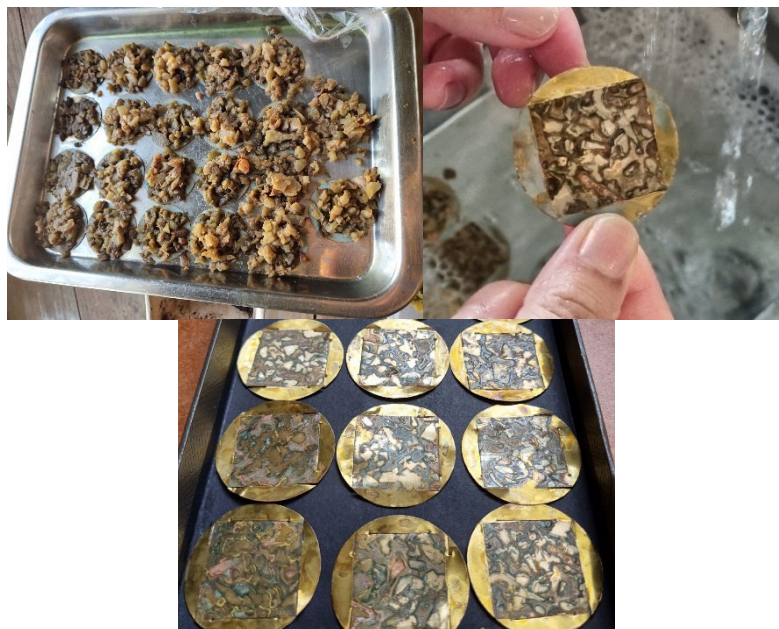
Figure 15 Brass Modules in Rose Apple Solution after 7 days, Cleaning, After Cleaning (Author, 2024)
