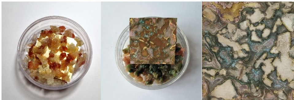
Figure 8 Process of Rose Apple Solution Patination on 0.1 mm-thin Brass Sheet (Author, 2024)
