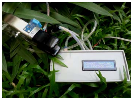
Figure 3 Photograph of the portable photosynthetic sensor
