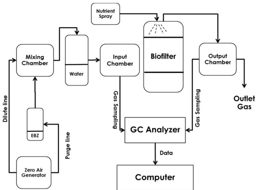
Figure 1 Schematic of the biofilter experimental system
