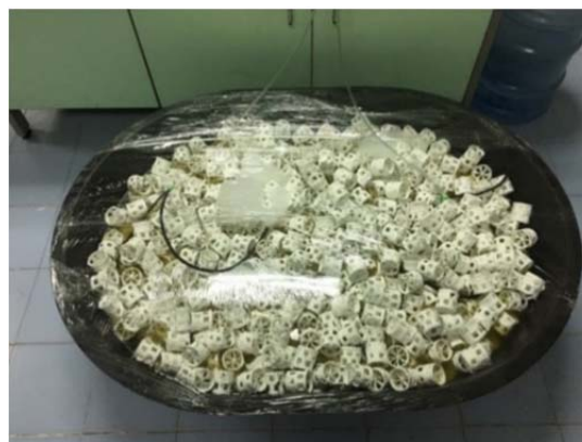
Figure 1 Pall ring plastic media fixed with bacteria on the surface
