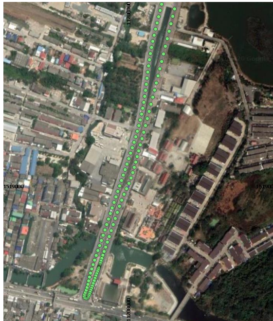
Figure 7 Showing the same area as Figure 6. The green dots is the positions processed by Wichiencharoen and Santitamnont [1]. Continuous computed positions, when the vehicle was moving southward, can be seen. The result of the old data was different from the new data (in Figure 6)
