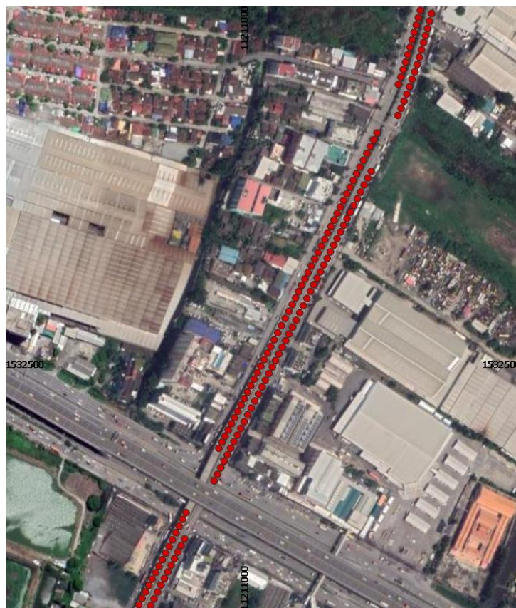
Figure 4 Showing a section of an enlarged map of Figure 3 . The red dots were positions of the MMS processing result at every one GPS second. Google Satellite was plug-in as the background
