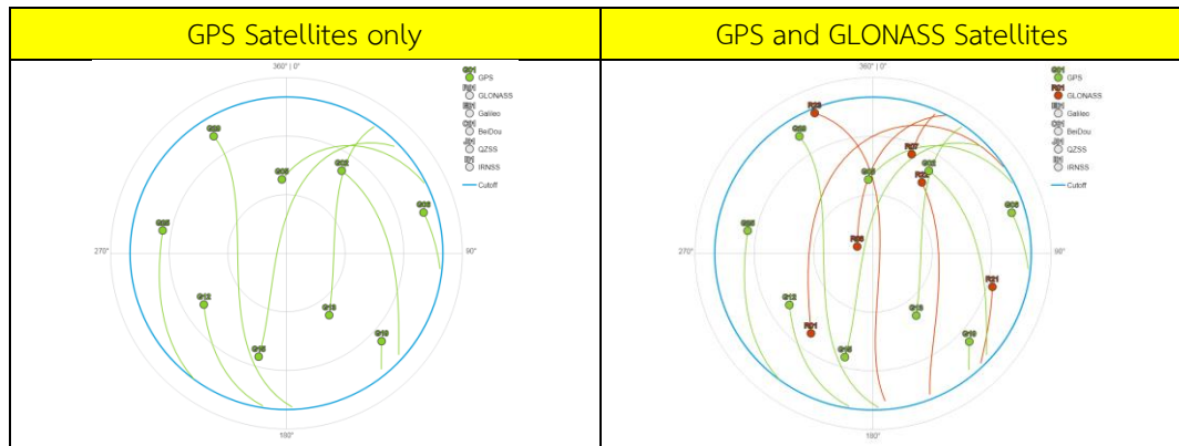
Figure 5 Sky plots at 13.00 hrs. (local time) on May 21, 2019, using [9]. Lines were paths of satellites for the next 6 hours
