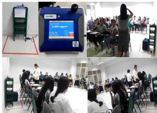
Figure 2 The sampling of PM2.5 by a DustTrak meter in classrooms
