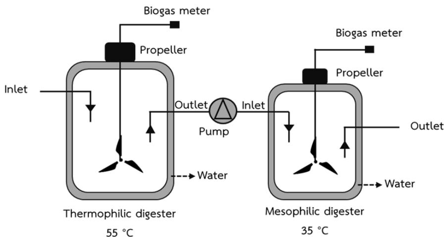
**Figure 1** Diagrammatic of temperature phase anaerobic digestion reactor
