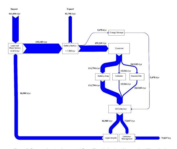
Figure 2 Diagram showing the material flow of lead in lead acid battery by MFA method
