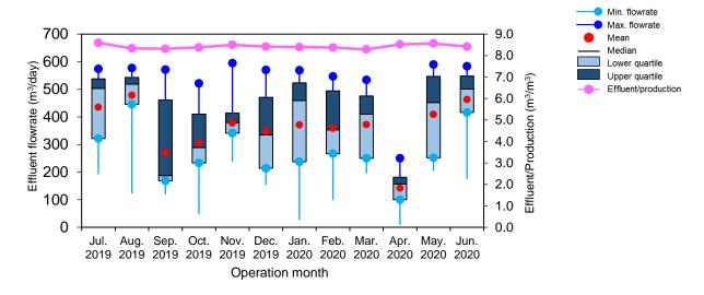
Figure 3 Box plot of UASB effluent flowrate
