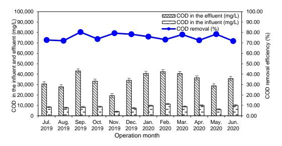
Figure 4 COD in the influent & effluent of UASB and removal efficiency
