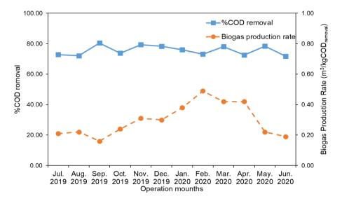
Figure 5 COD removal and biogas production rate
