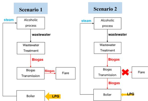
Figure 2 Schematic of 2 scenarios considered in this study
