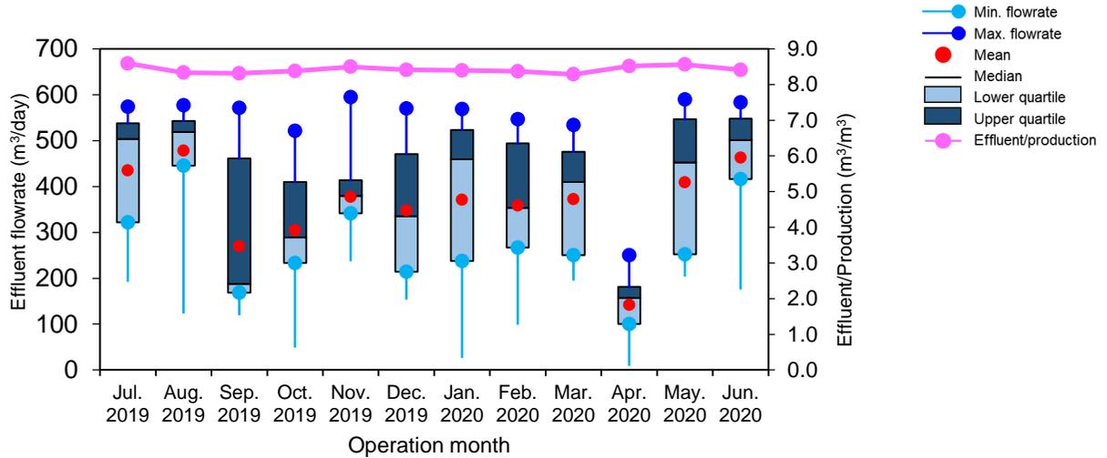
Figure 3 Box plot of UASB effluent flowrate
