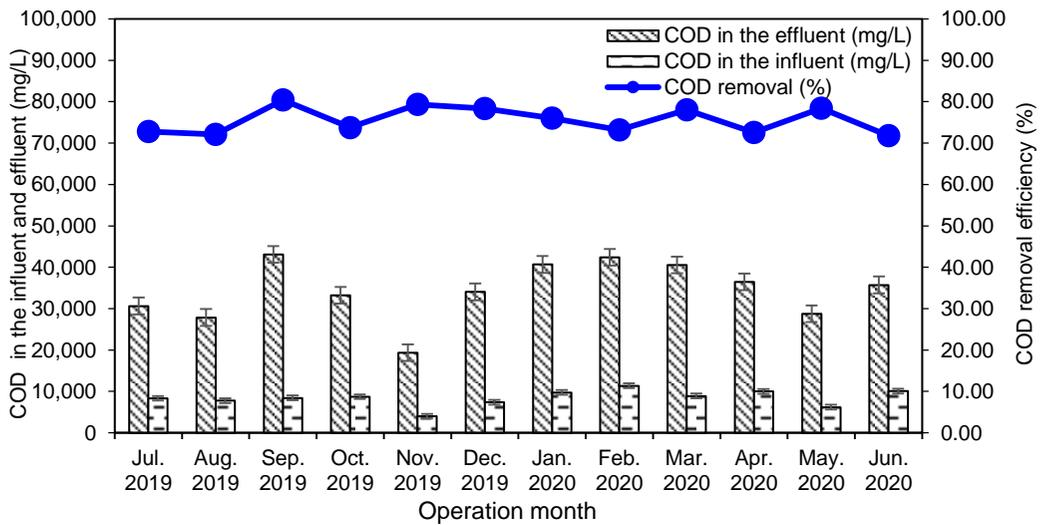
Figure 4 COD in the influent & effluent of UASB and removal efficiency
