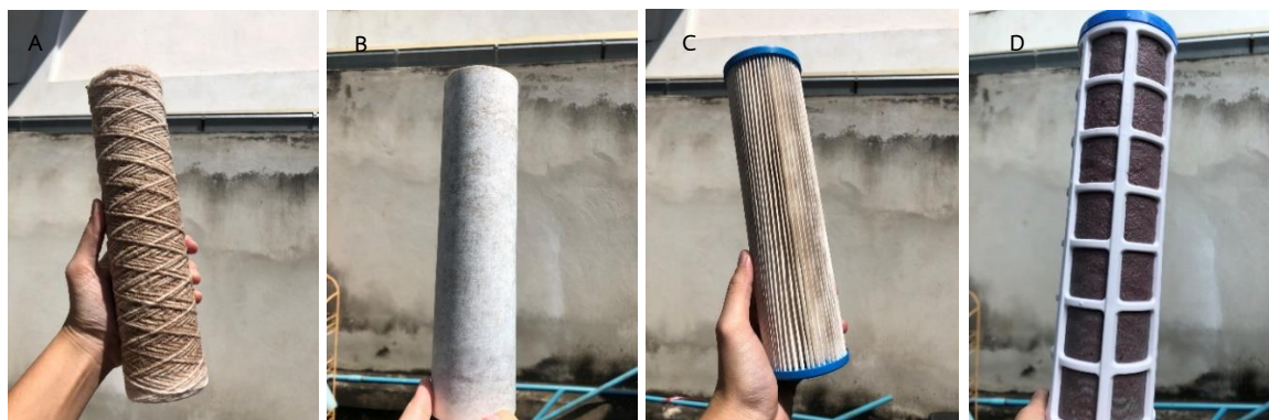
Figure 4 Filters that have been used to filter microplastics in washing machine waste once A: Yarn Filter Cartridge 5 \mu\text{m} , B: Polypropylene Smooth Filter Cartridge 5 \mu\text{m} , C: Polypropylene Pleated Filter Cartridge 5 \mu\text{m} , D: Stainless steel Filter Cartridge 40 \mu\text{m}
