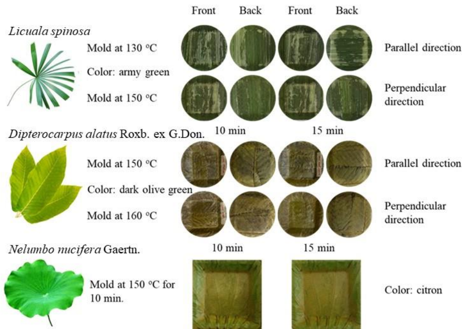
Figure 2 Characteristics of the three types of leaves, experimental conditions, and color of each leaf bowl
