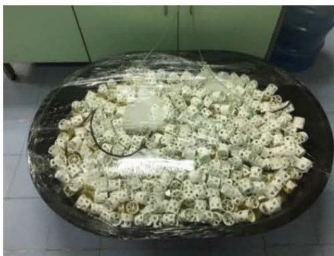
Figure 1 Pall ring plastic media fixed with bacteria on the surface
