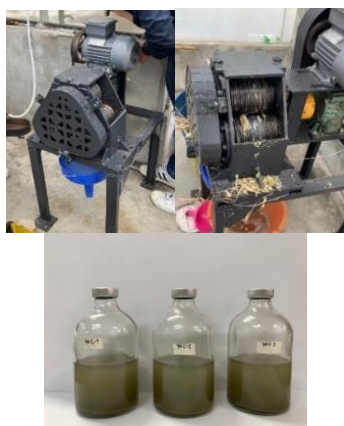
Figure 1 Cold screw press for produce extract Napier grass (A) and Napier grass extract age >90 days in serum vials (B)
