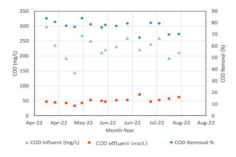
Figure 4 COD content in influent, effluent, and removal in SBR
