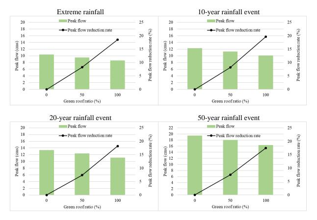
Figure 6 Variation of peak flow and peak flow reduction rate
