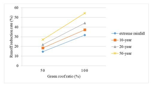
Figure 3 The impact of rainfall return period and green roof ratio on runoff reduction rate
