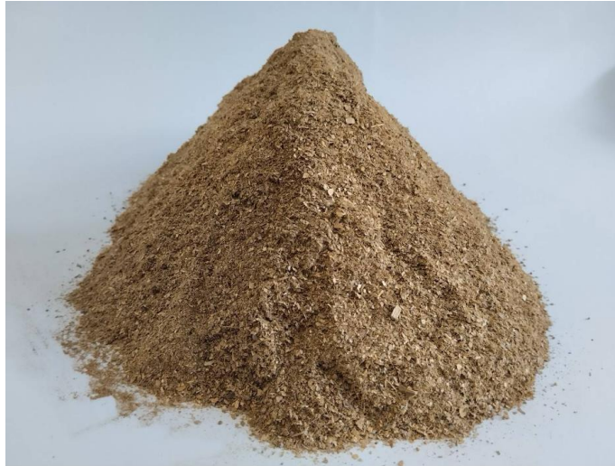
Figure 1 Preparation of leaf waste: leaves were sun-dried, ground using a semi-fine shredder, and dried again prior to forming
