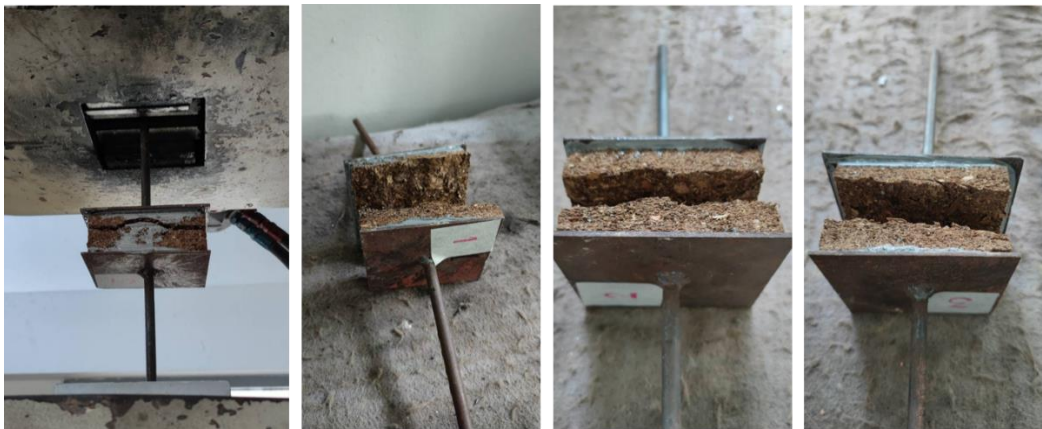
Figure 3 Tensile strength measurements of composite panels from the leaf waste.
