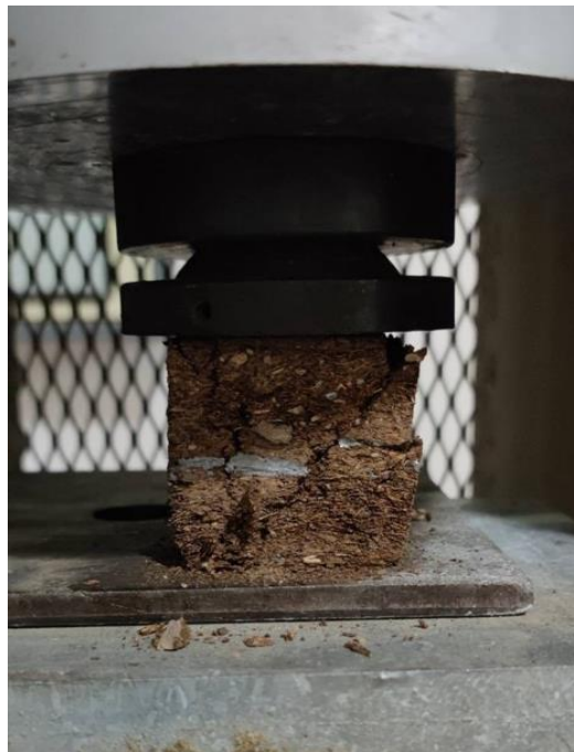
Figure 4 Compressive Strength test of composite panels from the leaf waste
